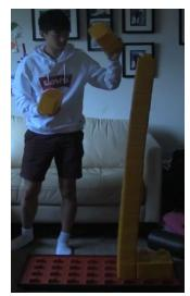
What we found was the the "shield" did not in fact help the blocks stack higher. We were only able to place 13 block before the stack gave out. this was <u>two blocks</u> less that of the original test. This further supported our theory that the distribution of weight factored in with the flexibility of the foundation resulting in smaller stacks.
