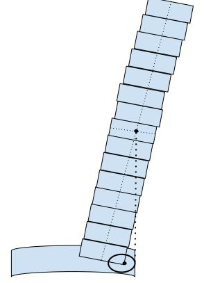
Due to the flexibility, the blocks are put at an angle. This causes the center of gravity to go over the tipping point much earlier than if the stack was in the middle. This is important because while dragging the foundation, the inertia of the blocks will naturally make them tip.
