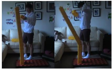
What we found was that the stack fell over in the direction it was away from the foundation center. To further test this theory, we placed the stack in the center. What we found was that the stack had gone to its highest yet; we were able to place a total of 18 stones.
