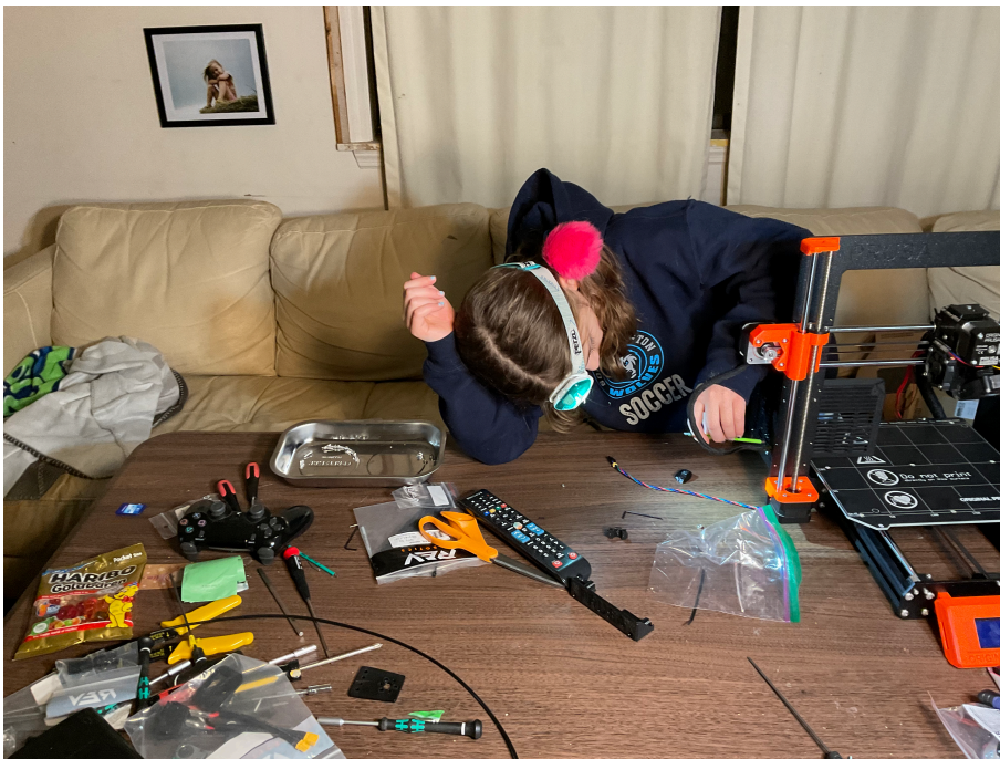
12/12/22 Fitting the Build Plate
